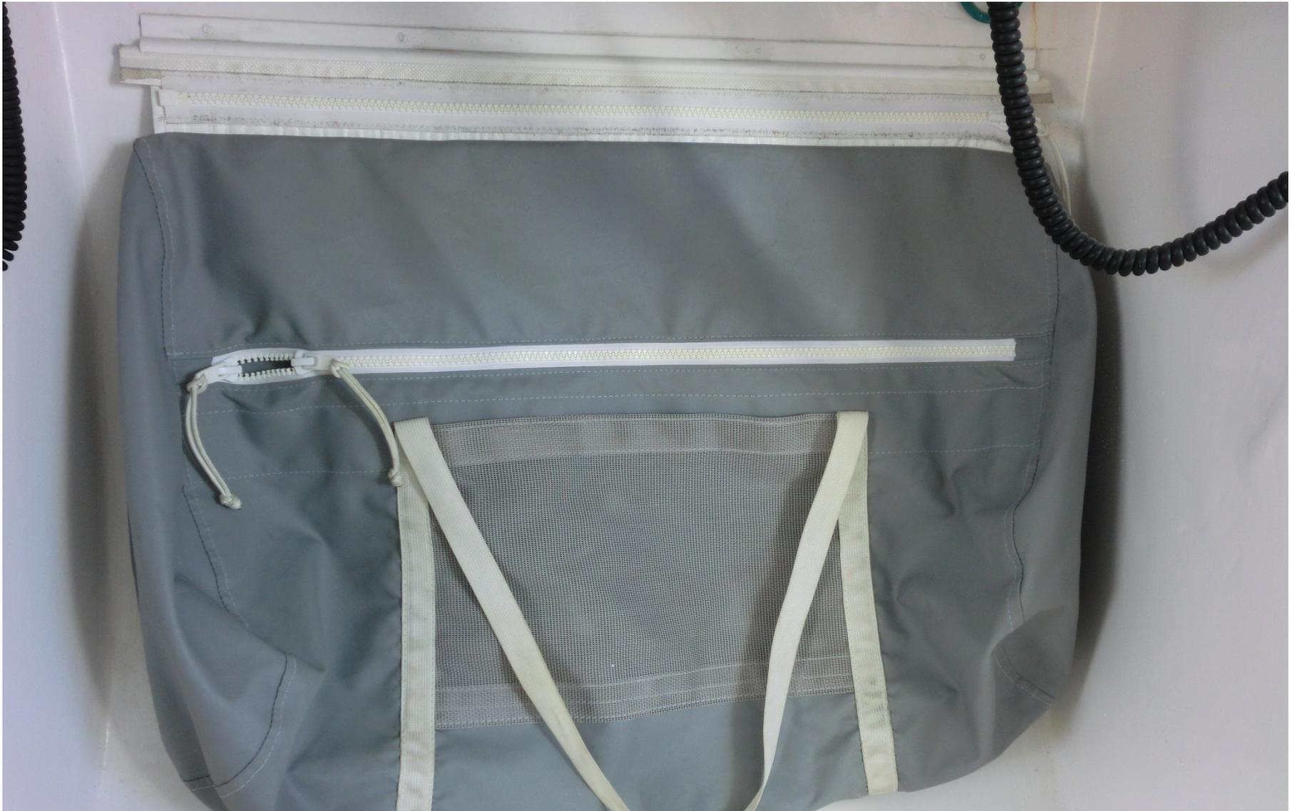
California Condor: Duffle Bags attached with zippers and awning tracks
